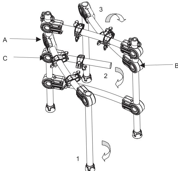
2. Put the long cymbal tube/short cymbal tube/L shape pad rod into the drum stand.
